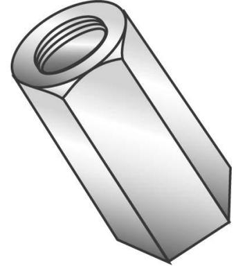
*A double chamfered hex nut used to join two externally threaded parts.*
