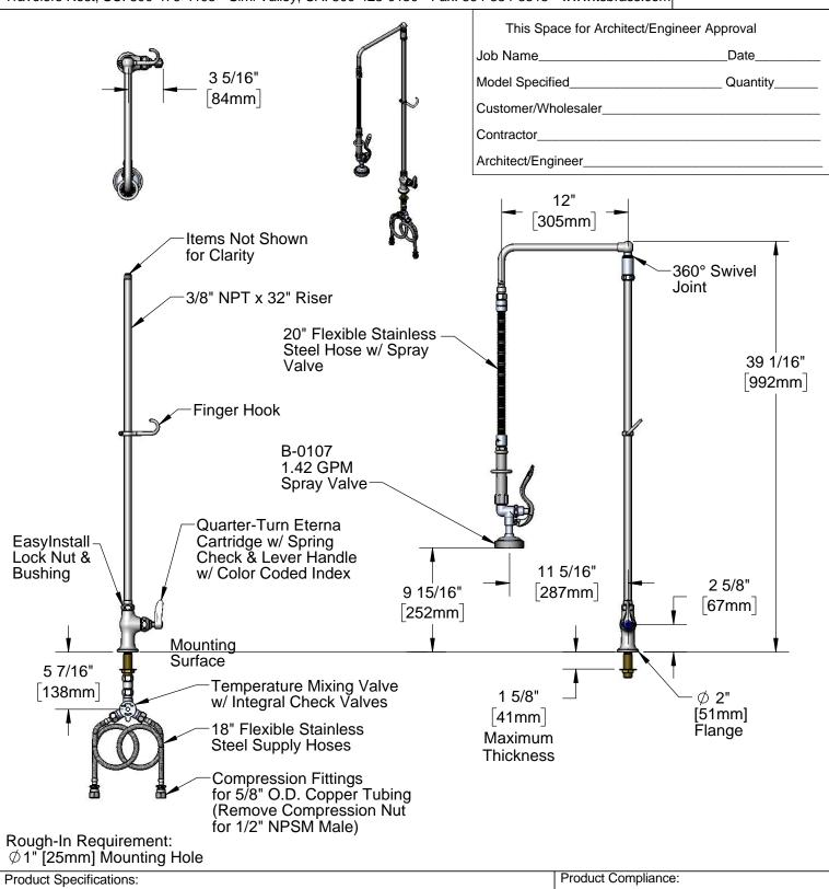
Single Hole, Single Temperature Deck Mount Mixing Faucet, Quarter-Turn Eterna Cartridge w/ Spring Check, Lever Handle, 12" Overhead Swivel Arm, 20" Flexible Stainless Steel Hose, 1.42 GPM Spray Valve, Temperature Control Mixing Valve w/ Integral Check Valves & 18" Flexible Stainless Steel Supply Hoses w/ 1/2" NPSM Male Inlets
