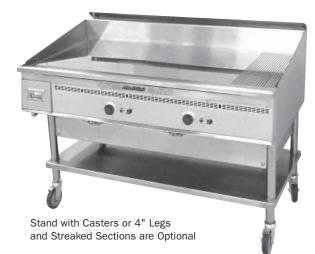
The Keating MIRACLEAN® Griddle is designed to provide maximum performance with many benefits to the operator. The mirror surface is achieved in a special eight step process. High input burners rated at 30,000 BTU/hr. for natural gas are mounted every 12" to ensure performance and recovery allowing the operator to use zone cooking for different products.
