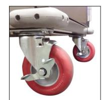
**HEAVY-DUTY PERFORMA CASTERS...** 5" diameter industrial grade casters with non-marking red rubber cushioned tread. Rust resistant Delrin bearings with all axles and raceways equipped with Zerk grease fittings. Long lasting and easy rolling, yet durable enough to withstand rigorous cart wash programs. Two fixed and four swivel casters with brakes for easy maneuvering.
