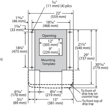
Recommended counter opening size 9" (229 mm) x 12" (305 mm) for utilities and tubing. Opening can be located anywhere within the shaded area.
