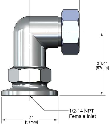
Drawn Checked Approved **Product Specifications:** ARH DMH **JHB** 1/2" NPT Female Inlet 90° Flange Asm, Chrome Polished Brass Date: Scale: 1:1 06/26/09
