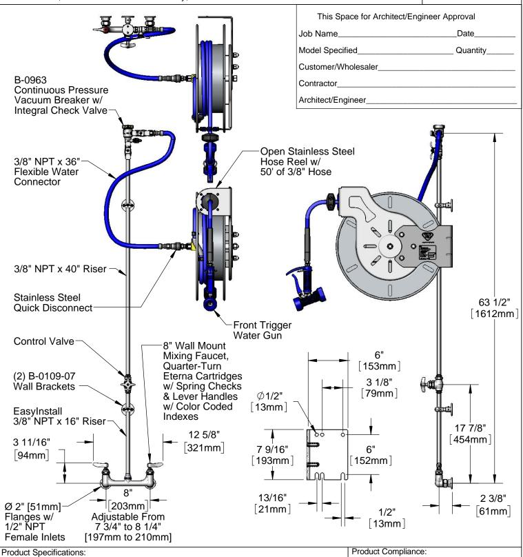
Open Stainless Steel Hose Reel w/ 50' of 3/8" Hose, Blue Front Trigger Water Gun, Vacuum Breaker, 3/8" NPT Flexible Water Connector, 8" Wall Mount Mixing Faucet & Control Valve
