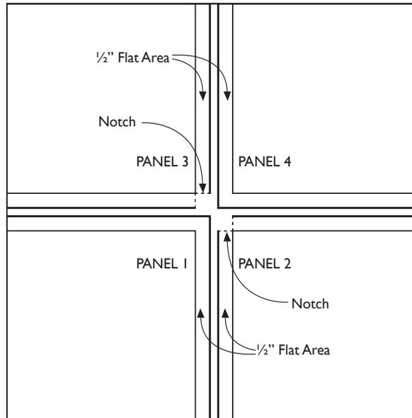
5. Carefully apply the adhesive to the ceiling (or wall for 2' x 2' wall applications) and lay up your first tile applying pressure as you hold it. (If installing a tile with protective masking, you can remove it at this step of the installation. Make sure the tile is straight before you continue with the next one.
