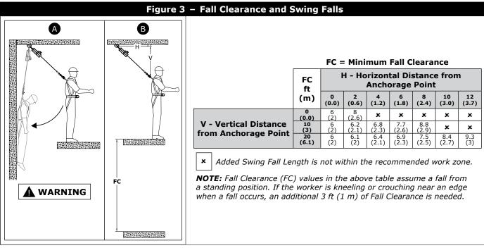
**NOTE:** The clearances provided above assume the fall occurs from the standing position. If the worker is kneeling or crouching an additional 3 ft (1 m) of clearance is needed.
