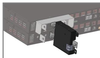
The compact size of the ICT 100A Redundant Isolation Module allows it to be mounted directly to the output bus bars of two 1RU ICT Platinum Series or Pro Series power supplies, saving valuable space and reducing the need for extra cabling.
