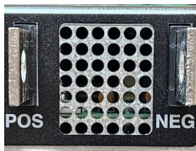
Figure 16. The DC Output Bus Bars
