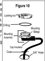
Using a spanner wrench or long nose pliers to hold the Mounting Assembly
