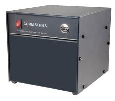
The ICT Backup Series combines backup batteries, power supply, and enclosure, all pre-assembled into an integrated compact solution. The power supply provides DC power to the radio while charging the internal battery, then if AC fails it will automatically and seamlessly transfer the load to the battery for up to 8 hours (depending on radio model and current draw).
