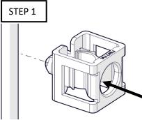
APPLY PRESSURE THROUGH HOLE TO SPREAD INNER SPRING CLIPS
