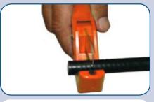
Straighten cable. Use RDCUTTER-S, applying even pressure around cable while rotating tool around cable to cut off cable squarely.
