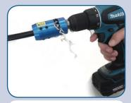
Actuate drill to remove jacket and expose the center conductor. Then remove cable from tool.
