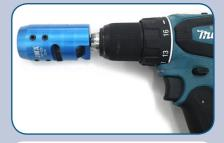
Attach prep/strip tool to drill. Be sure you are using an SP-12S tool.
