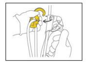
The ROLLCLIP Z pulley may be used as a directional point on the upper attachment point of the ASCENSION handled rope clamp, for short rope ascents. Gate opening on the non-pulley side facilitates installation on the ASCENSION.
